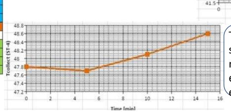
This is the first laboratory work with solar collectors, we had to wait 15 minutes from the start of the experiment and fix the parameters every 5 minutes.
