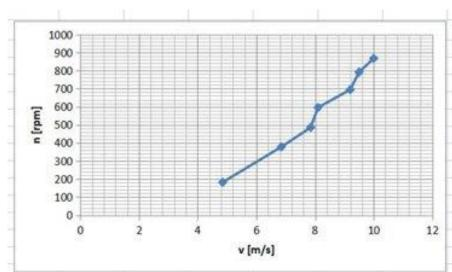
We increased the speed of the turbine and noticed the following dependence: the faster the turbine rotates, the higher the speed of the wind, the faster the fan rotates.
